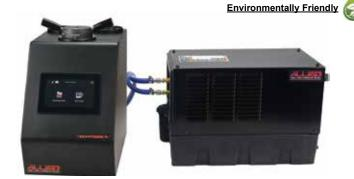
The recirculating coolant system connects seamlessly to the **TechPress 3x**™ for standalone or "green" operation. The 3-gallon system circulates a unique coolant that effectively cools the mold assembly after the curing cycle. This not only saves water (~ 12 gallons per cycle), it eliminates problems associated with hard water deposits in the coolant system inside the press, which can cause clogging over time.
