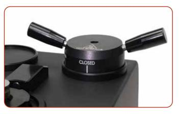
Bayonet holding tray protects the die from damage between cycles.
